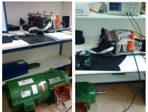
Fig. 15. Experimental Setup. The-level Three-phase NPC inverter and motor drive.
