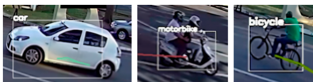
Fig. 3. Vehicle detection with Non-Maximum-Suppression.
