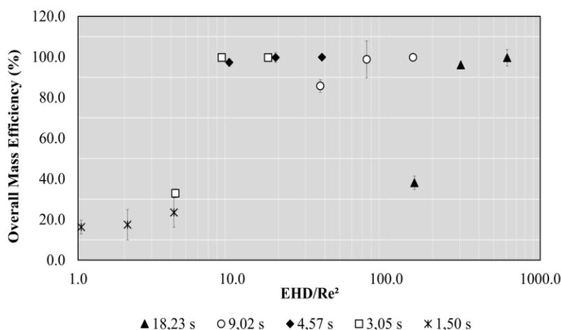
Fig. 5. Overall efficiencies of the tests in relation to  $EHD/Re^2$  for different residence times
