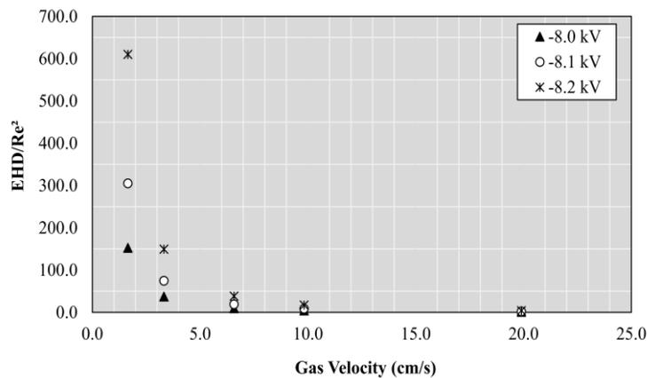
Fig. 3. EHD/Re<sup>2</sup> ratios obtained in the tests
