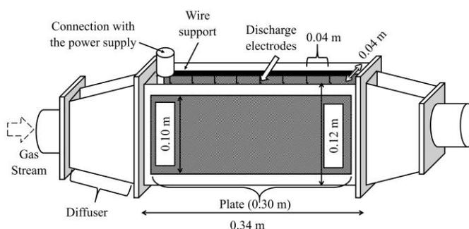
Fig. 2. Scheme of the ESP used in the tests
