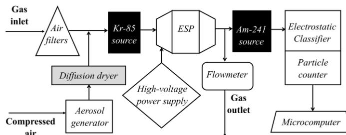
Fig. 1. Scheme of the experimental system
