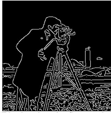
Edge detection using Canny method
