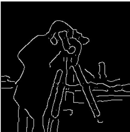
Extracted edges using canny method
