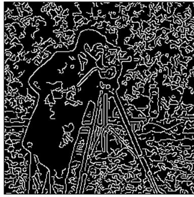
Edge detection using Canny method
